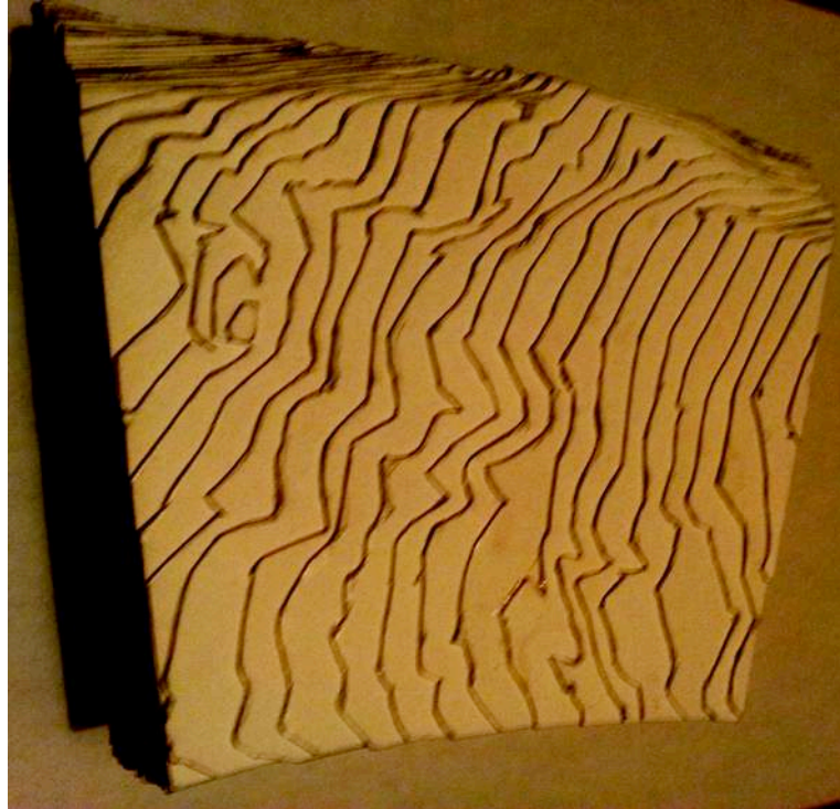
3-D relief map with 2' contours of 203 Kupaia Place, Lot 30 Kawela Plantation. Note steep cliff face on top (north) and gully traces of sheet erosion throughout. Non-cliff altitude variation is typical of all lots. Below Lot 30 north view, lot corners: red circles.
